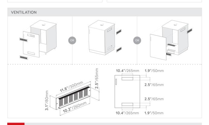
PLEASE NOTE It is essential to allow for two ventilation points when installing FRIIA. Vents are not supplied. Where possible, we recommend removing the back of your cabinet.
